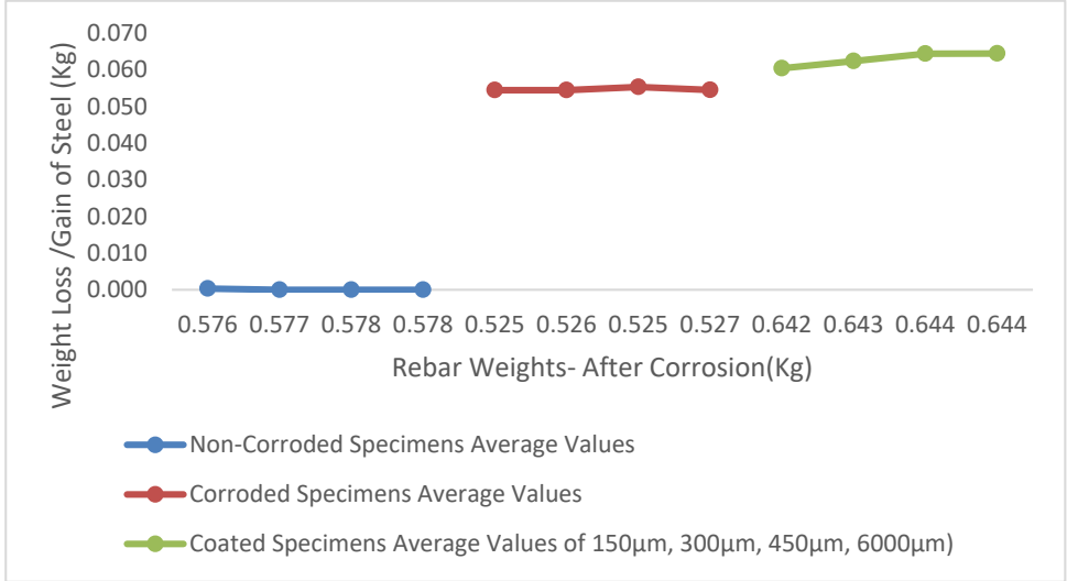
Figure 6: Rebar Weights- after Corrosion versus Weight Loss /Gain of Steel
